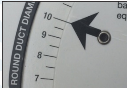
Figure 23 A 10 in. Duct Size Selected on the English Units Side of the Ductulator
