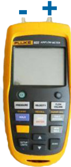
Figure 5 Digital Gauge Positive and Negative Connections
