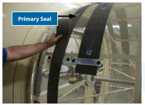
Rotate drum cage(s) and wrap primary seal around circumference of drum cage until seal overlaps. Pull seal tight.
