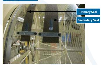
Attach one end of the primary and secondary seal to drum cage using supplied holding brackets and plastic rivets.
