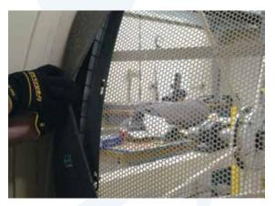
Work secondary seal over seal stops towards plenum wall while manually rotating the drum cage(s).
