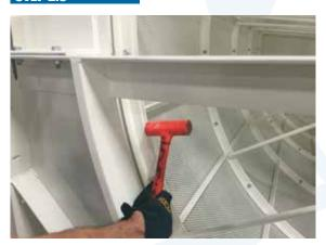
Adjust the height of the rigid seal stops by tapping them with a rubber mallet from the inside of the drum.
