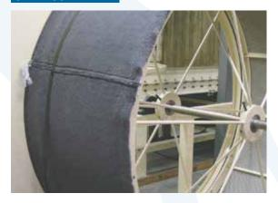
Wrap seal retainer holding band around circumference of drum cage section.
