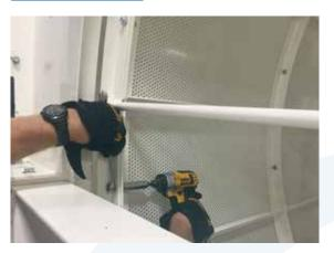
Loosen the bolts on the plenum cage section that are holding the rigid seal stops in place.
