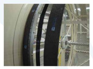
Using integrated hook and loop material, join ends of elastic retainer.
