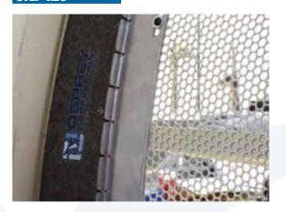
Primary seal is in correct position when entire seal is between seal stops and plenum wall, and one side of seal is in contact with seal stops.
