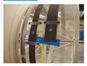
Butt primary seal ends together and attach remaining end to drum cage with holding bracket. Place non-stick backing material under seal ends.
