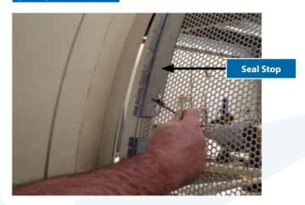
Attach flexible seal stops to drum cage with supplied hardware, bolted through the second available row of perforated holes in the drum cage.
