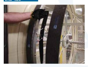
Temporarily attach one end of elastic retainer to outside of drum cage.
