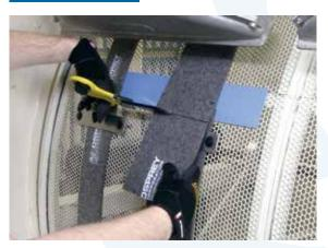
Cut secondary seal at new mark ensuring that the cut is perpendicular to the sides of the seal.
