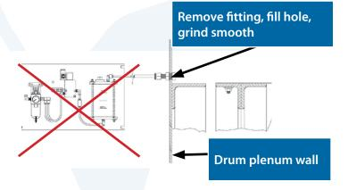
**NOTE** – If Auto-Lube assembly is installed on filter, disable and remove. Ensure fitting on plenum wall is removed and remaining hole is filled with liquid steel and ground smooth.
