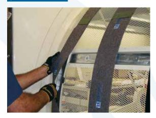
Remove holding brackets and non-stick backing material and work primary seal over seal stops towards plenum wall while manually rotating the drum cage(s).
