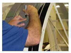
After hot glue has fully cured, center seal reinforcement over seal joint.
