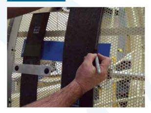
While the primary seal reinforcement hot glue is curing, rotate drum cage(s) and wrap secondary seal around circumference of drum cage until seal overlaps. Mark the location of overlap.
