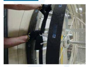
Rotate drum cage(s) and wrap elastic retainer around circumference of drum.
