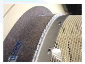
Secondary seal is in correct position when one side of seal is in contact with seal stops, opposite side of seal will be in contact with plenum wall.
