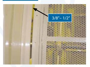
Align Drum Cage to plenum wall to obtain UNIFORM 3/8" - 1/2" [10 mm – 13 mm] gap.
