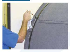
Install seal retainer holding band between plenum wall and seal stops. Seal retainer holding band should clamp around the drum cage angle ring, not the plenum wall angle ring (see drawing below).
