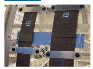
Butt secondary seal ends together and attach remaining end to drum cage with holding bracket.
