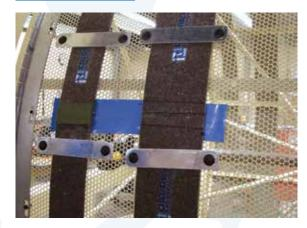
Mark the perimeter of the seal reinforcement.
