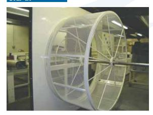
Install drum cage section(s), drum shaft, and drum drive. (If applicable)
