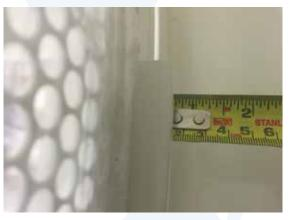
Continue adjusting the height of the rigid seal stops until they protrude 5/8" (16mm) from the outer surface of the drum cage section.
