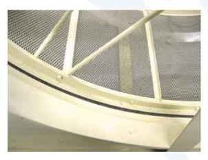
**NOTE** – Ensure drum cage angle ring and plenum wall angle ring are in good condition with no burrs or sharp edges. Grind smooth if necessary.
