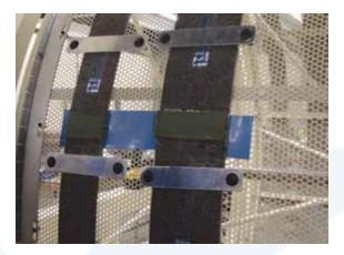
Quickly place seal reinforcement over the area covered with hot glue.
