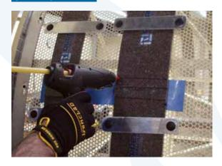
Apply hot glue to seal surface between seal reinforcement perimeter marks.
