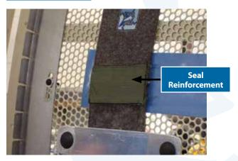
Quickly place seal reinforcement over the area covered with hot glue.
