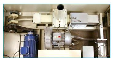
The inlet design includes a vacuum blower that assists material entering the heat and compaction chamber.
